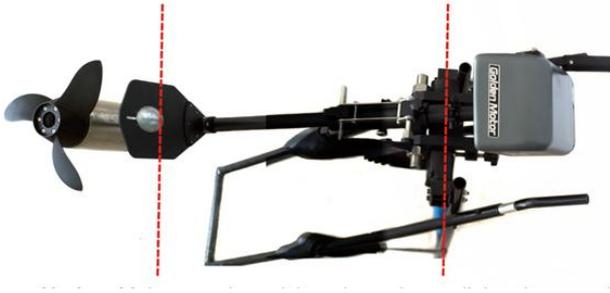
**Tilting down:** Pull the silver switch out, and tilt down the outboard slowly, then close the angle adjustment release handle.
